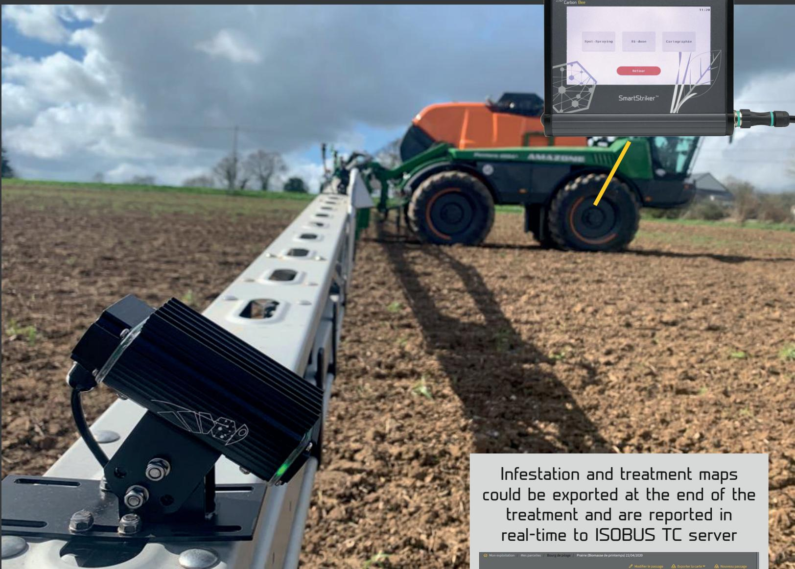
The Controller receives the information from the sensors and merges it to control the spraying and create the map in real time.
