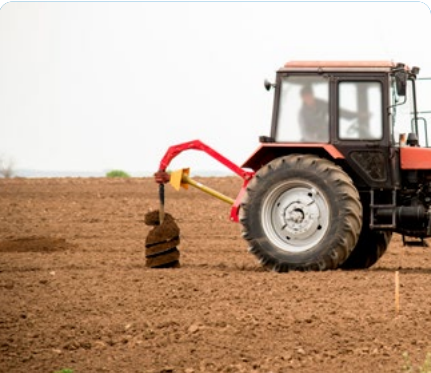
Post Hole Digging
